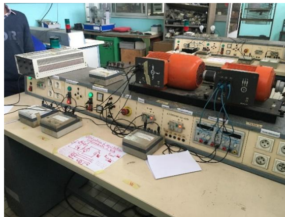
Figure 3. Measurement setup in a laboratory. The decision to place the sound level meter on a frame very close to the machine itself is well placed to avoid the influence of noise.
