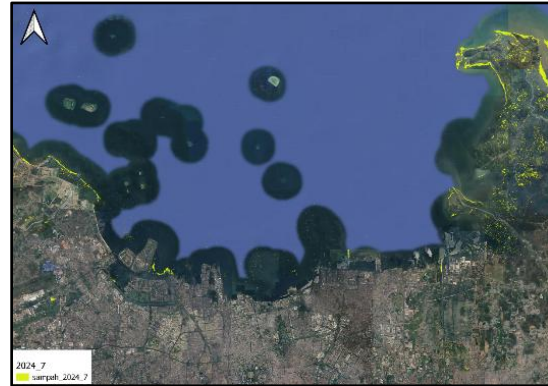
Figure 5. Detection results of floating debris using NDVI and FDI in July 2024.
